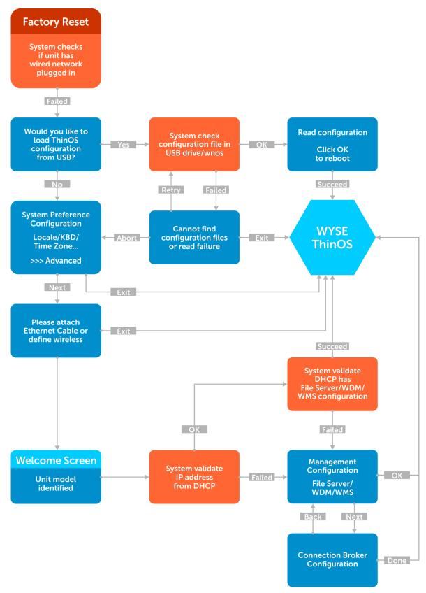
Figure 2. First Boot Wizard—network failure
