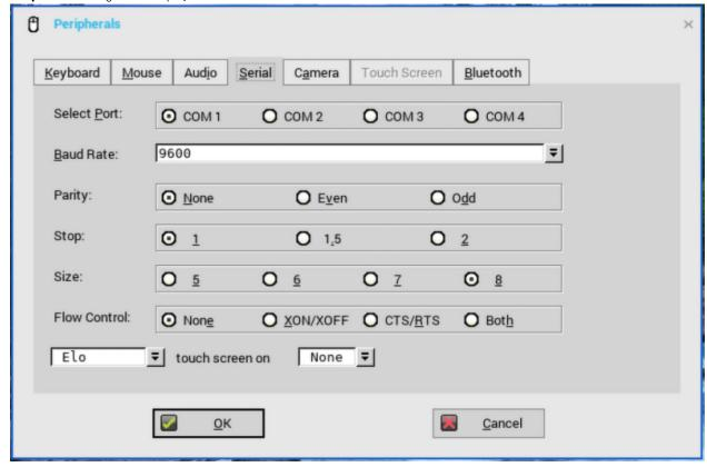
Figure 31. Serial tab
